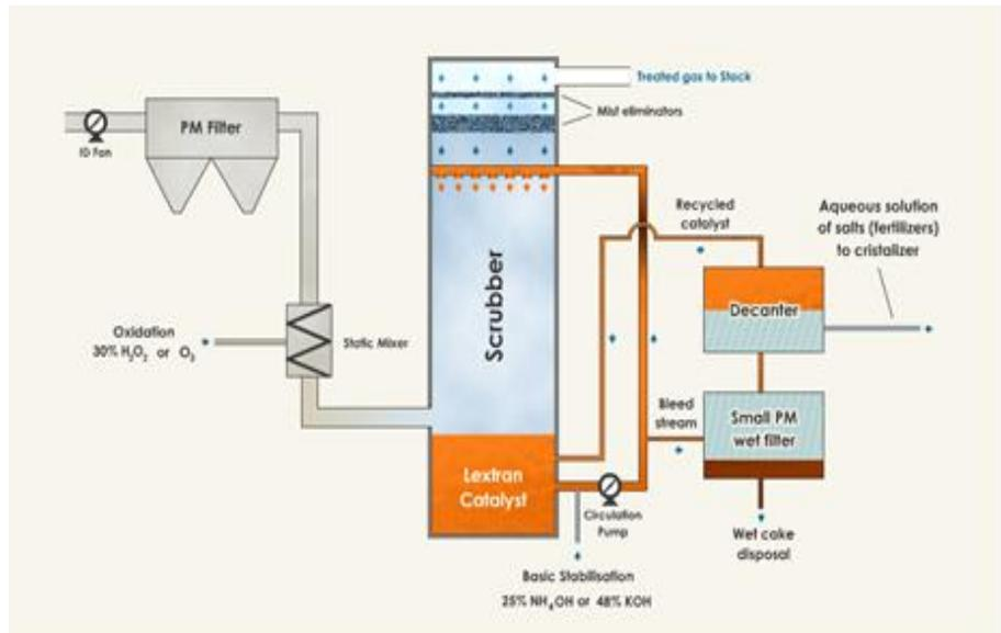
Figure 2. Schematic design of Lextran's WFGD-based operation. Removes NO<sub>x</sub> and SO<sub>x</sub> from flue gas and converts them into fertilizers.
