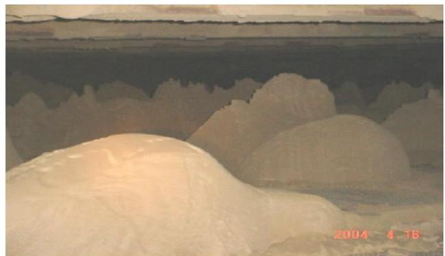
Figure 1. Ashes deposits on SCR catalyst surface
